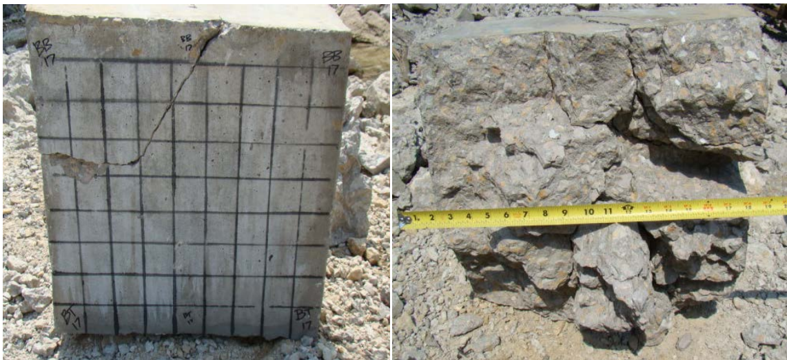
Figure 4.22: Block 17, back face and interior views after impact
