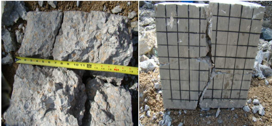
Figure 4.3: Block 1, interior and back face views after impact.
