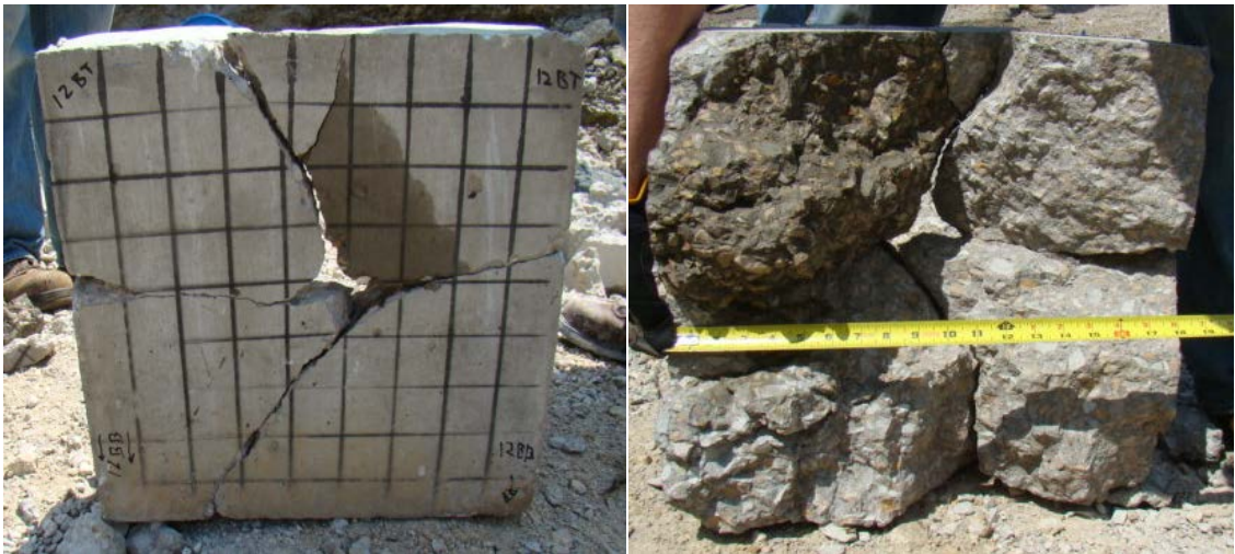
Figure 4.17: Block 12, back face and interior views after impact
