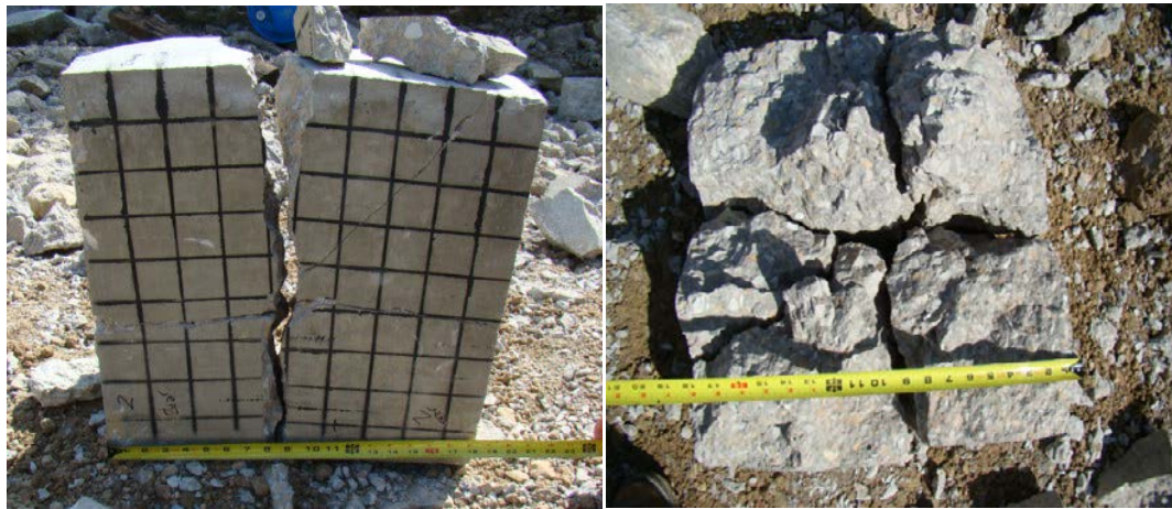
Figure 4.4: Block 2, back face and interior views after impact.
