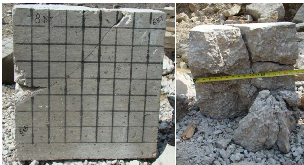
Figure 4.12: Block 8, back face and interior views after impact.
