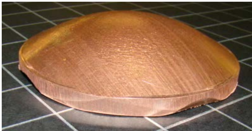
Figure 3.1: Completed flyer plate.
