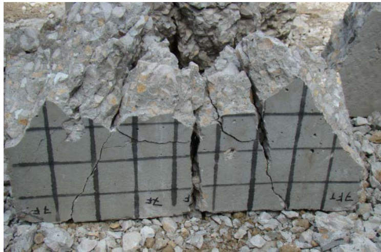
Figure 4.11: Block 7, front face pieces recovered after impact.
